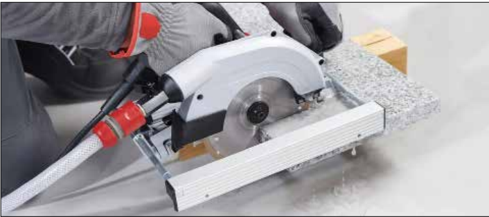
High-performance motor: extra-powerful, for cutting stone and milling joints
